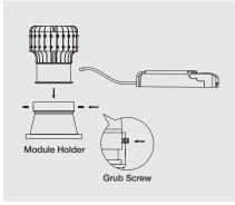
4. Grub screw to tighten between module & module holder and connect module to driver.
